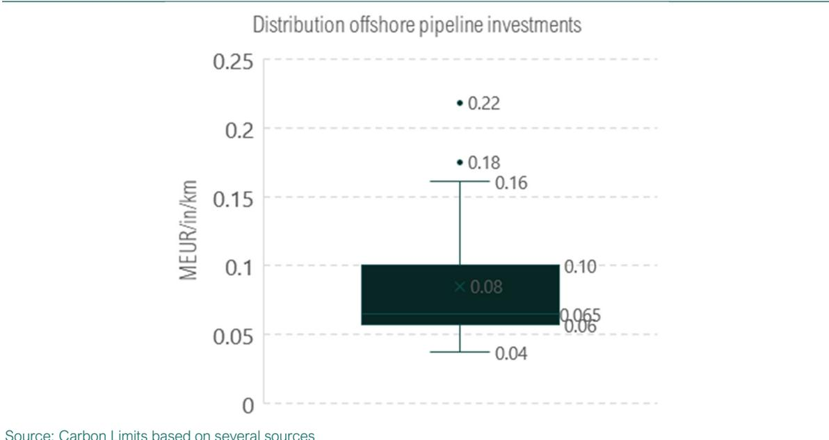
Figure 20 compiles 23 published costs of recently laid / designed pipelines offshore. The average of the costs lies at 0.08 MEUR/in/km and that 50% of the data lies between 0.06 and 0.10 MEUR/in/km. Some statistical outliers from the database of 23 data points can be found, at 0.18 and 0.22 MEUR/in/km. The reasons for this scattered data are associated to, among other things, landfall costs, vessels mobilization and demobilization.
